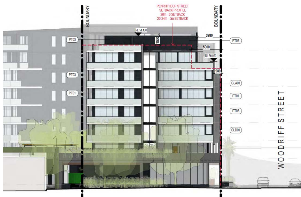
Figure 11 Southern elevation showing minor DCP breach relating to street setback profile
