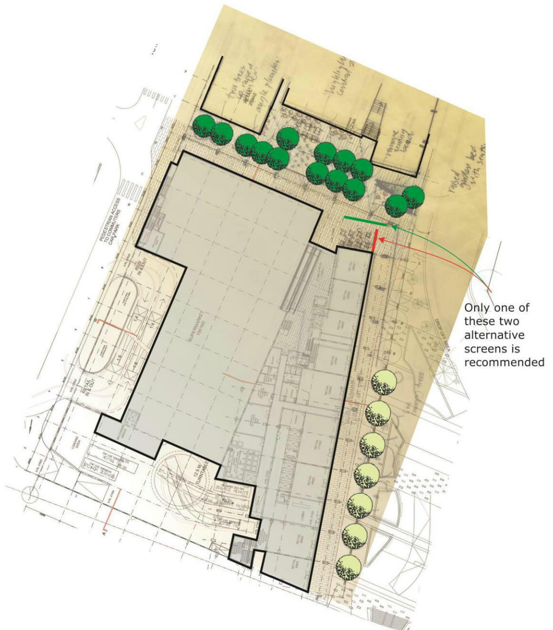
Figure 2: Recommended Treatments (Ground Level)
