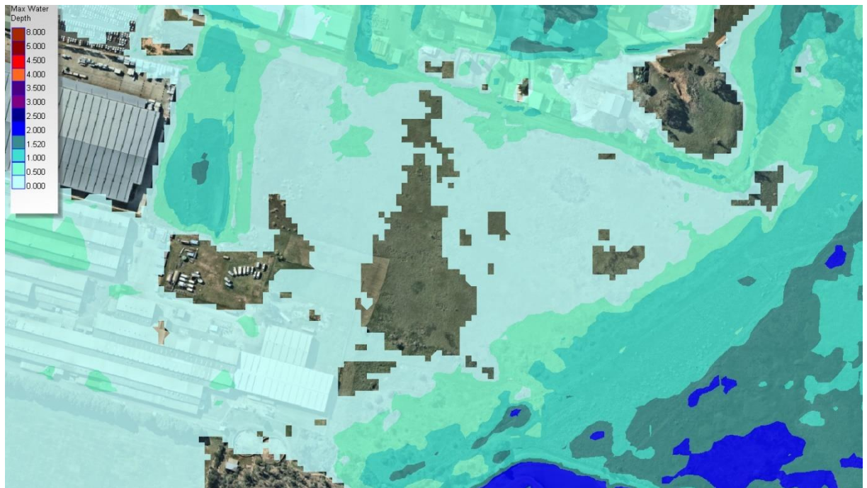
Figure F11 – 0.5% AEP Flood Depth – Pre-Development
