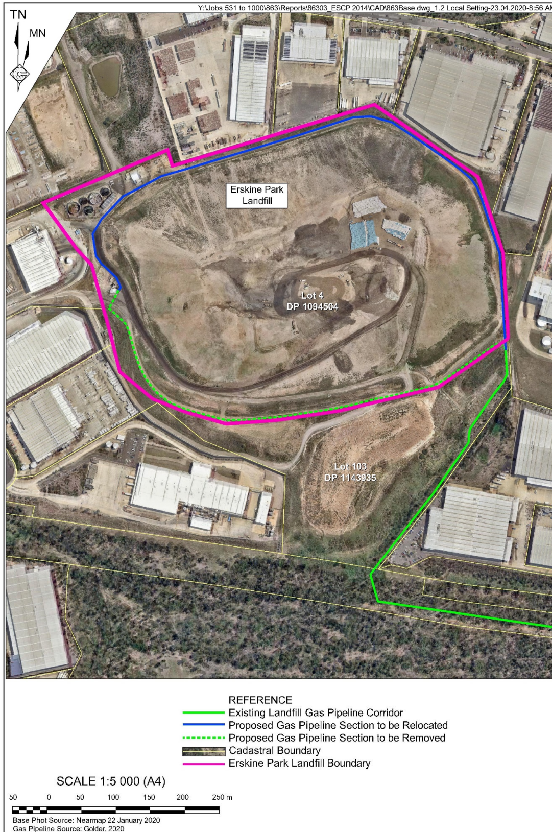
Figure 6 Proposed Relocated Landfill Gas Pipeline
