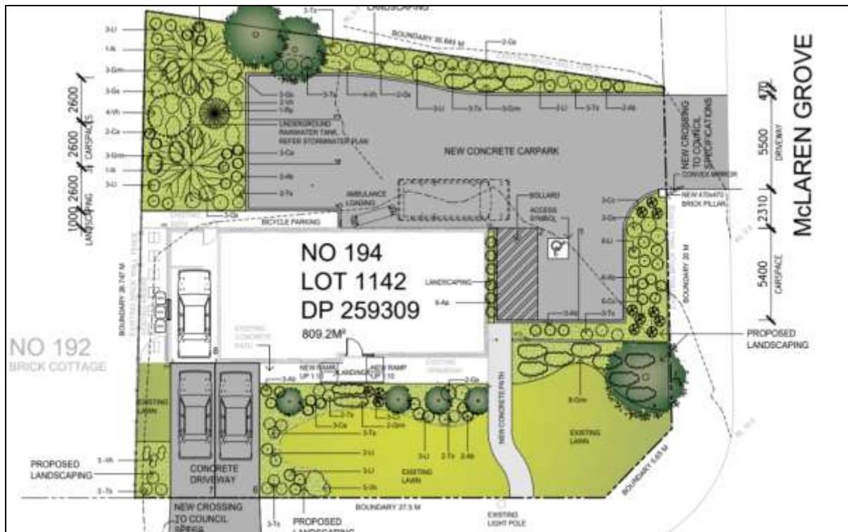
Figure 9: Proposed Site Plan including new rear carpark with bicycle parking. Source: Proposed Site Plan & Landscape Concept Plan, A1.2, prepared by BDAA Accredited Building Designer, 30 March 2021.
