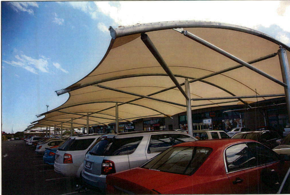
Figure 8: Concept image of proposed colour scheme. Galvanised steelwork Shade cloth: Beach Sand
