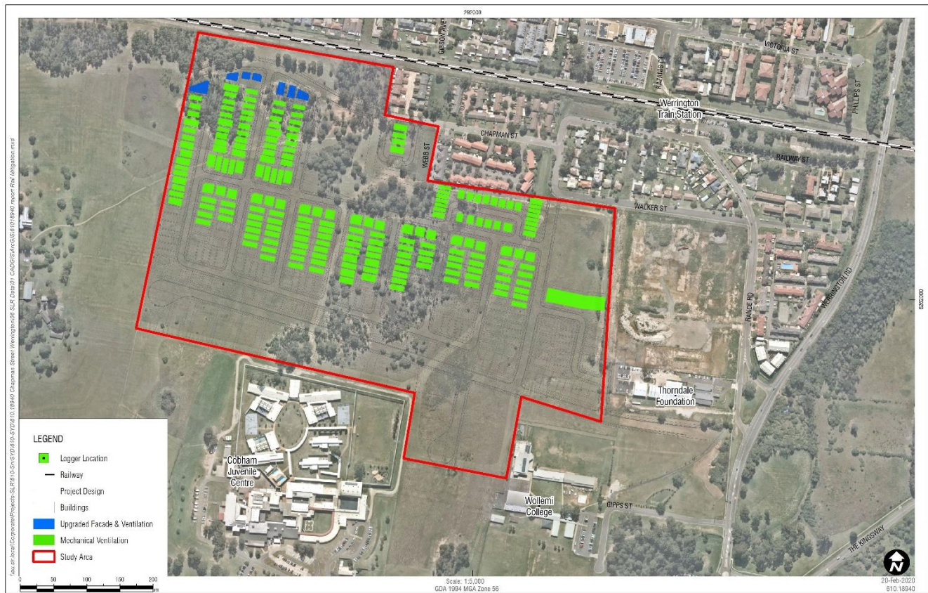
Figure 9 Indicative Locations for Upgraded Facades and Mechanical Ventilation – Existing Rail Noise
