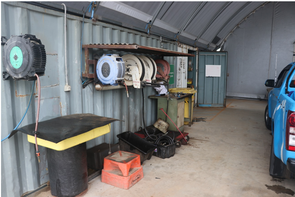
Photograph 10: View of interior of workshop showing lubricant dispensing area, with secondary containment tubs below.
